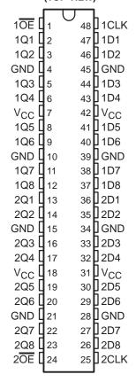
These devices can be used as two 8-bit flip-flops or one 16-bit flip-flop. On the positive transition of the clock (CLK) input, the Q outputs of the flip-flop take on the logic levels at the data (D) inputs.
